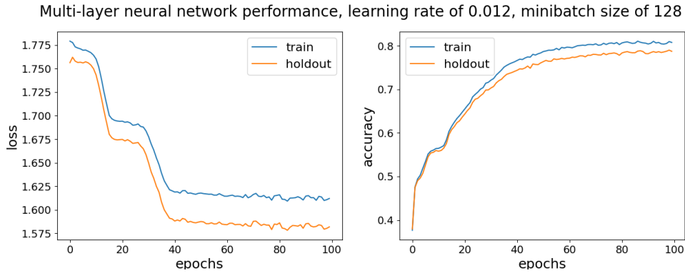
Figure 2: Performance of neural network consisting of 2 hidden layers of 50 nodes and tanh activation and a softmax output layer. Utilized a learning rate of 1.2e-2 , momentum gamma of 0.9, and no regularization. Trained using stochastic gradient descent of mini-batch size 128 over 100 epochs with early stopping.
